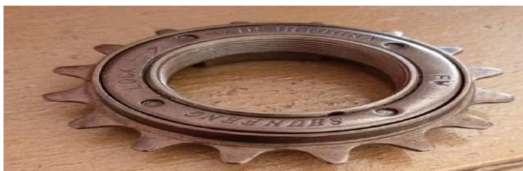
Figure 9. The freewheel moves in one direction
