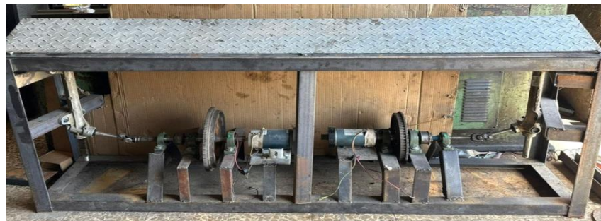
Figure 15. The speed bumps with its two generation systems.
