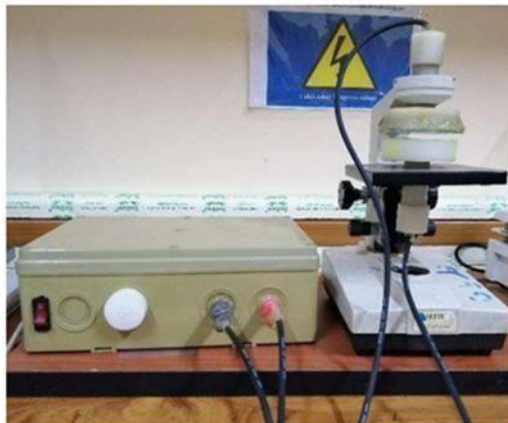
Figure(1) :Schematic of a two-electrode electrode position cell
