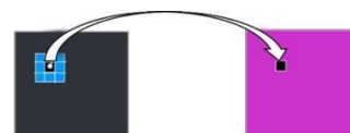
Figure 3: Convolution process generating new information from neighboring information in the input image [10]
